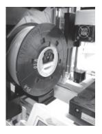
First open the release arm and then pull out the filament with spool axle rings. Arrange it properly for later use.
