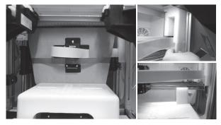
Before using this printer, please first remove the fixed materials from the printing module and printing bed. Switching on the printer's power without removing these fixed materials may damage the machine.
