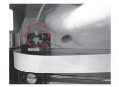
2 After the extruder has been adjusted, insert the guide tube into the extruder.
