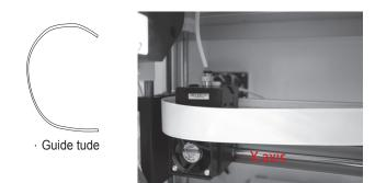
Before installing the guide tube, turn off the printer and move the extruder to the far left-end of the X-axis. If not done otherwise, the print quality will be affected.
