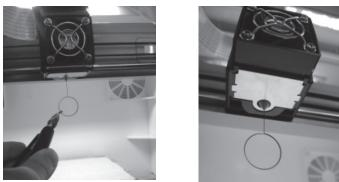
3.Hold the cleaning wire with the pliers, and carefully pass the wire through the nozzle openning.
