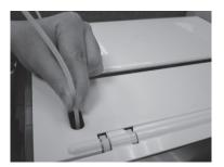
3 Direct the guide tube from the tube movement area out of the machine and then insert the other end of the filament tube into the feed module tube port.
