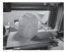
4.Remove the printed object when the printing has finished and the print bed has descended.The bed tape is reusable and it can be replaced when it's worn.
