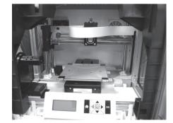
6 Remove the securing styrofoam next to the print bed.
