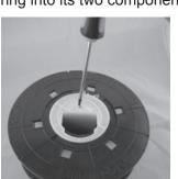
Insert the filament spool axle ring components to either side of the filament spool, and use a cruciform screwdriver to tighten and secure the rings to the axle to complete the installation of the filament spool axle rings.
