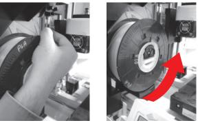
6 Pull out a section of the filament and insert it into the feed port.
