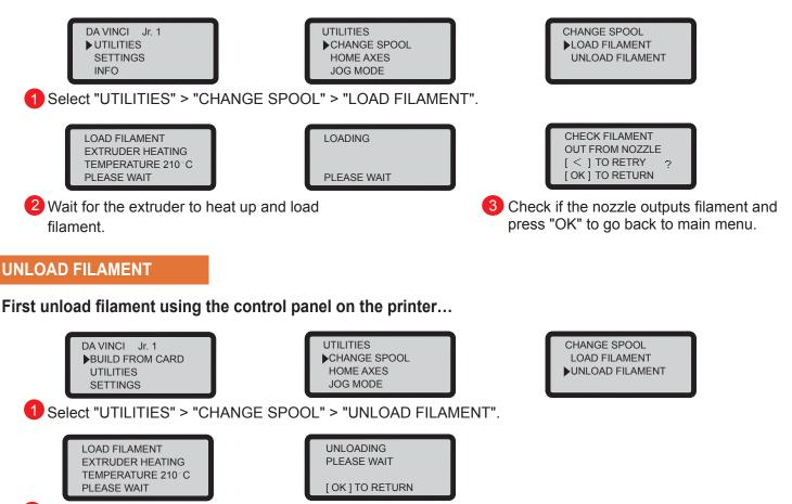
2 Wait for the extruder to heat up and unload filament. Press "OK" to pull out filament.
